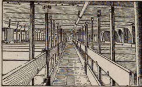
Fig. 139. Fittings of ocean transport for carrying cattle or horses. (Adapted from Bureau of Animal Industry Report, 1900.)
